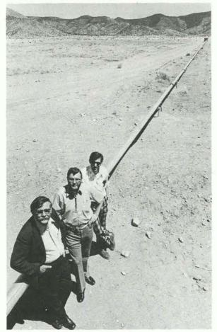
Laser strain seismometer
